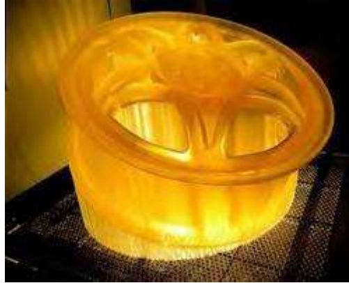
Figure 2 Component made by the SLA process suspended on support material which is attached to the build area.
